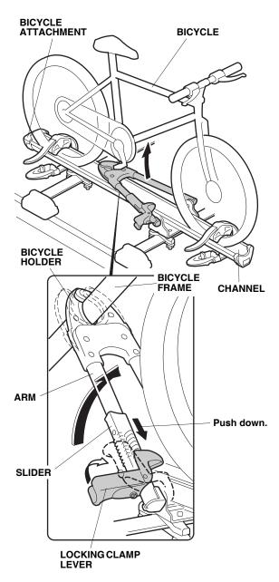
11. Push up the locking clamp lever to secure the bicycle frame.
